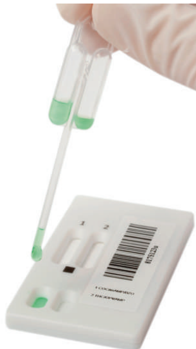
The illustration shows a pipette with a defined fill volume and a multi-test cassette.
